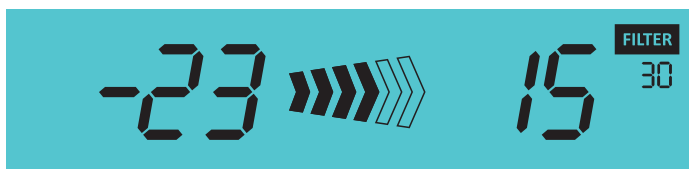
Figure 6. LCD display when the device is under manual control and filter replacement schedule is drawing near Error: Reference source not found
