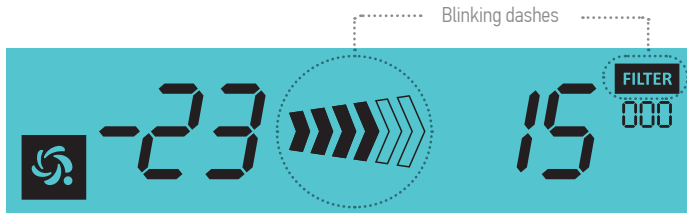
Figure 17. Configuration of filter replacement alert schedule
